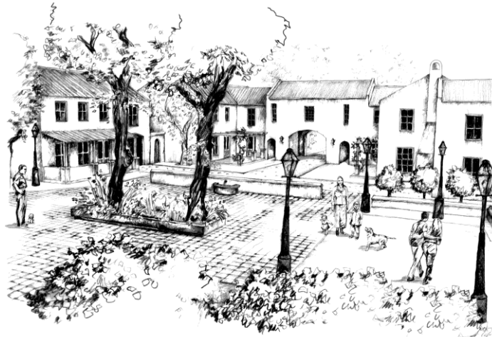
Figure 1: Illustration of homogenous architectural language, landscaping elements and typical courtyard formed by linking buildings together to achieve edge continuity. The urban design principle of integrated bridging is illustrated by the “poort” over the road that links buildings and defines the street edge.
