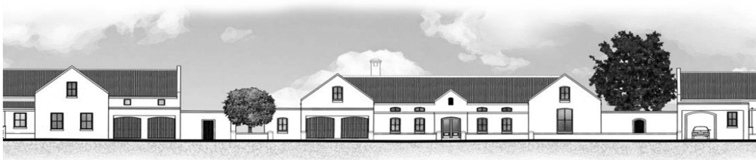
Figure 14: Illustration of linking elements used to connect individual houses and create edge continuity.
