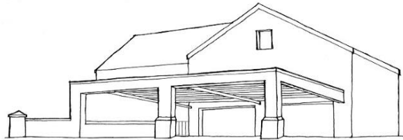
Figure 11: Garage doors screened from view by a coachman's entrance and timber pergola behind a horizontal parapet wall.
